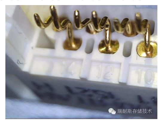
4. Male connector has to involve buffer design as well, both internal and external structure are clearly from below 2 angles:
